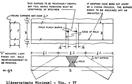
V = Width of the Surface of the Weld
