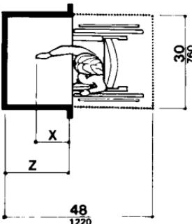
NOTE: x shall be  $\leq$  25 in (635 mm); z shall be  $\geq$  x. When x < 20 in (510 mm), then y shall be 48 in (1220 mm) maximum. When x is 20 to 25 in (510 to 635 mm), then y shall be 44 in (1120 mm) maximum.
