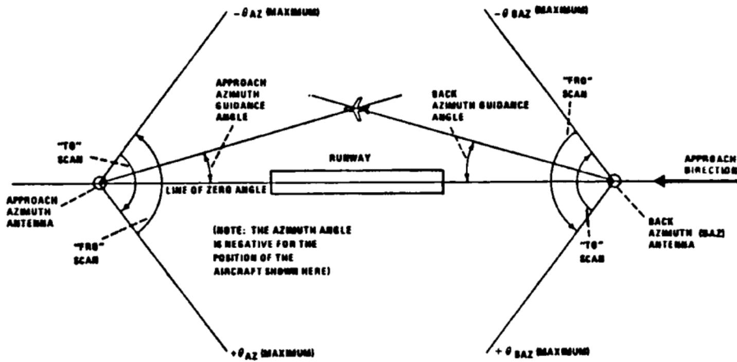
Figure 12. Azimuth Guidance Functions Scanning Conventions
