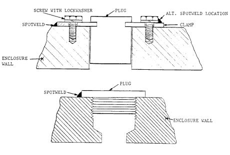
WELD (OR BRAZE) MAY BE ON PLUG, CLAMP, OR FASTENING
