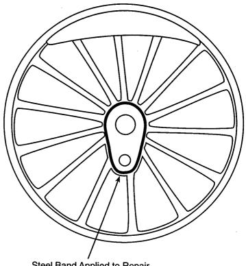
Steel Band Applied to Repair Cracked Wheel Hub
